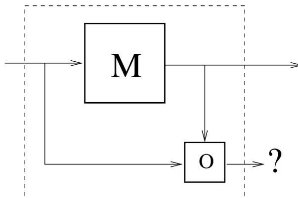
FIG. 3 – The observer technique. M is the program to be verified, o is the program which expresses the property to be verified on M.
