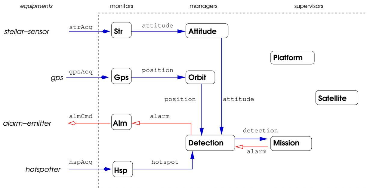
FIG. 1 – Simplified functional architecture of the Flight Software.
