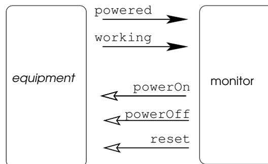
FIG. 2 – Control and state signals exchanged between an equipment and its monitor.
