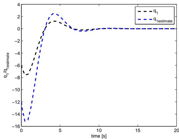
Figure 7: Convergence of the estimated state  $\hat{q}_1$  to its real value  $q_1$
