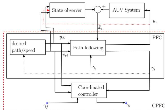
Figure 3: Coordinated path-following control system architecture
