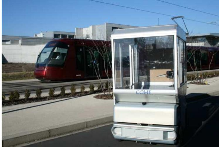
FIG. 9: RobuCab vehicle with the embedded camera.
